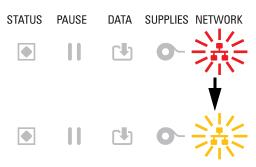
DATA SUPPLIES NETWORK The light flashes red while the printer associates with the network.
